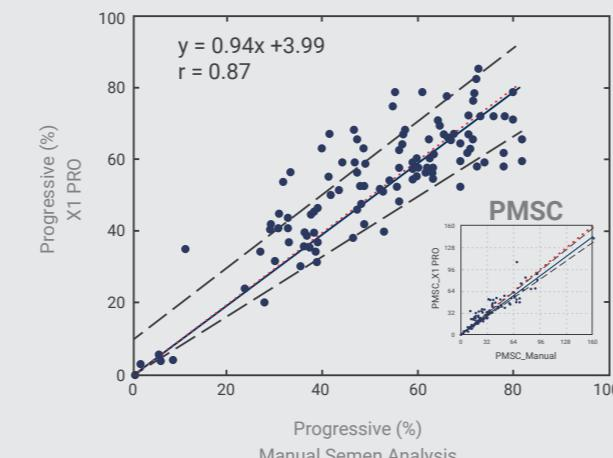
Comparison of progressive motility results between LensHooke™ Analyzer and a manual microscope method ( $n=100$ ). As shown below, the correlation of progressive motile sperm concentration (PMSC)  $r = 0.94$ .
